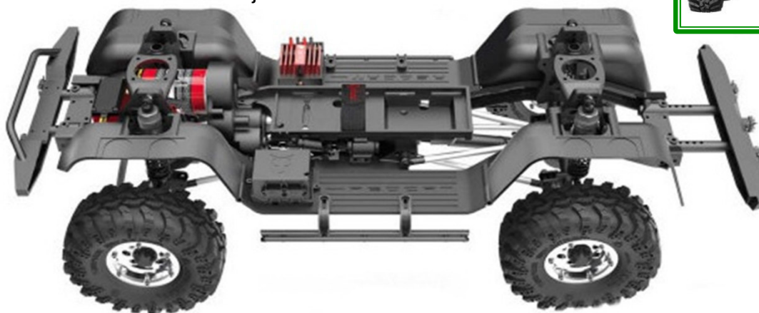
Portal axles with metal gear cover
